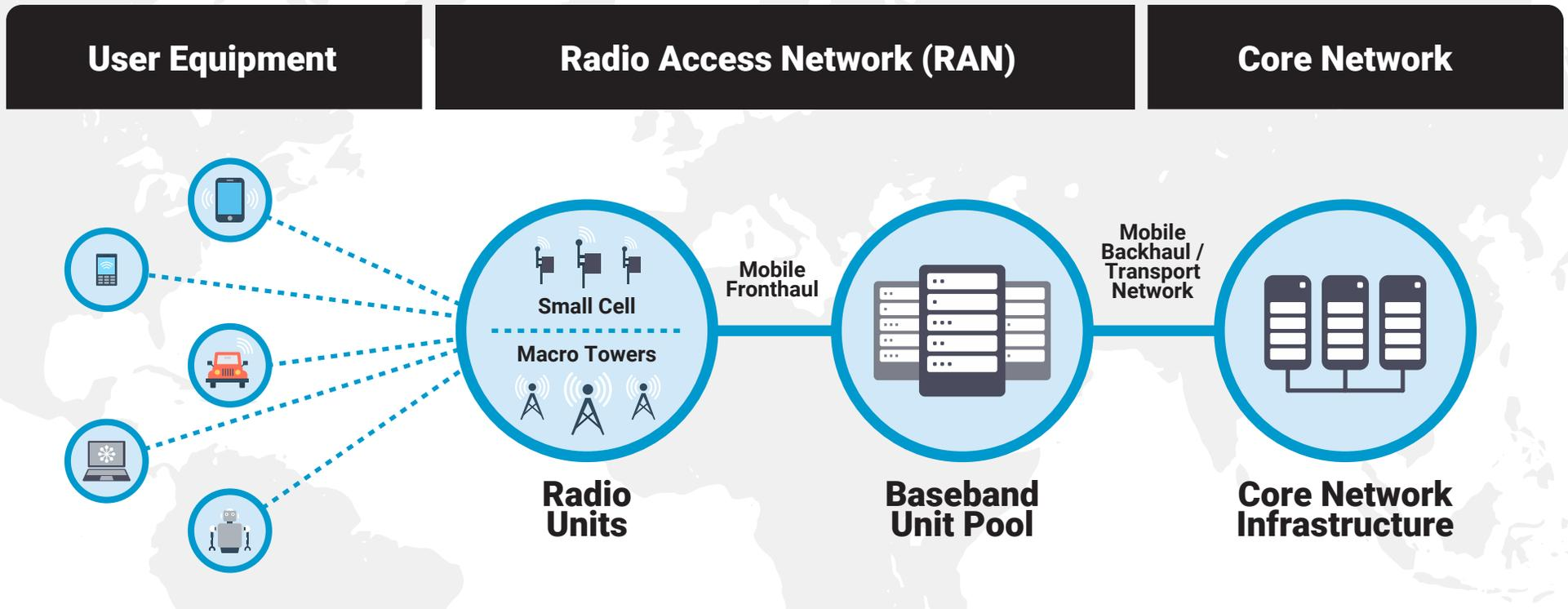
Devices such as smart phones, computers, and Industrial Control Systems (ICS) generate data that is then transmitted to a base station, small cell, satellite, or Internet Exchange Points (IXP). Compromised devices may collect user data and impact local networks and systems, but are unlikely to impact the larger communications network.
