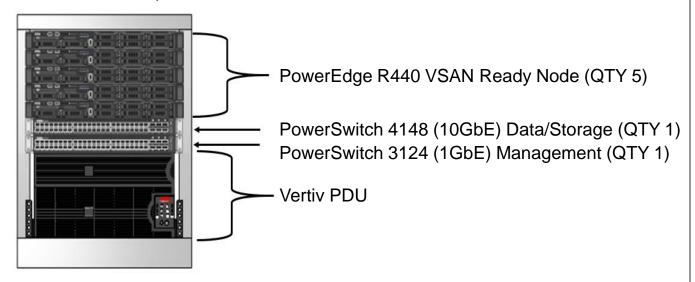
The ICAM POC Stack provides the necessary hardware and software for an organization to validate the functionality of the solution to meet their identity solution requirements.
